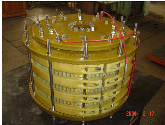
Figure 5. Overview of 100 kJ SMES HTS magnet.
