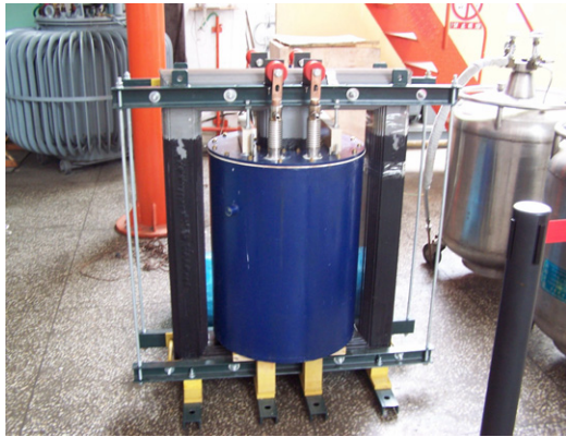
Figure 2. 45kVA single phase HTS transformer.
